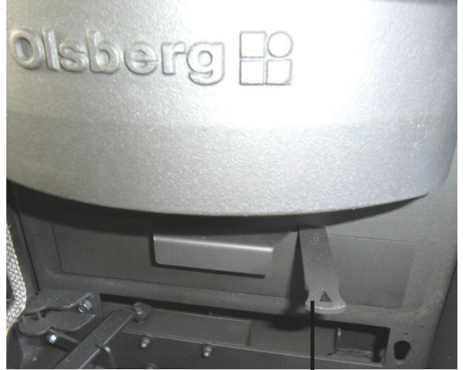
Operating lever for the fire grate
