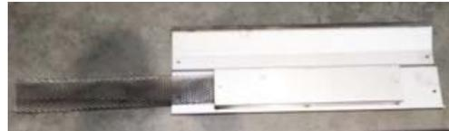
Slide a new wire mesh into the baffle cover every year
